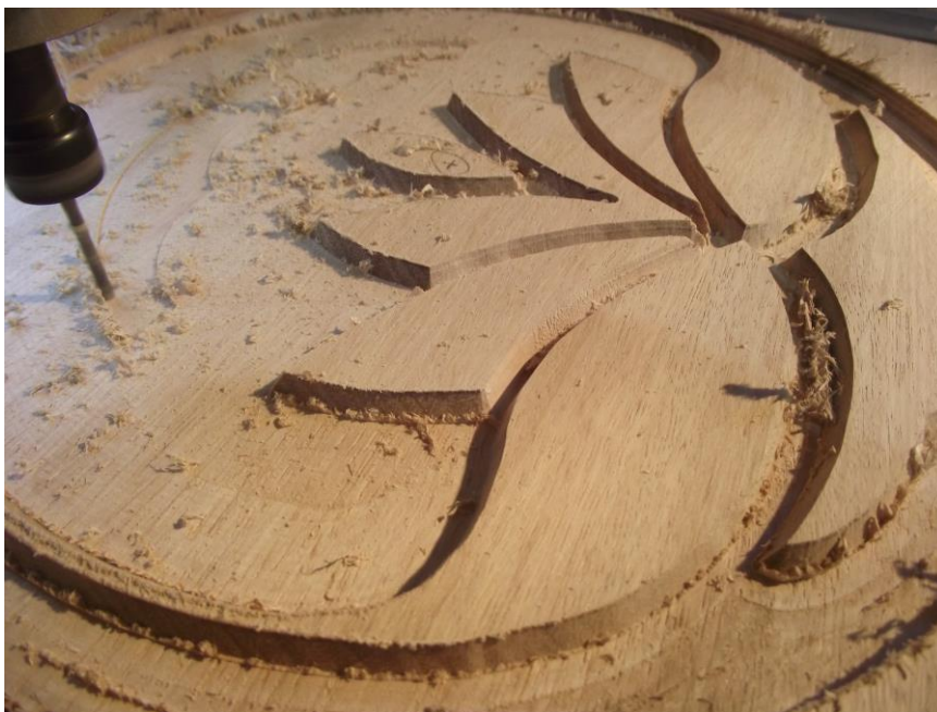
Figure 18: Clearing the Inlay with a pocket MOP
