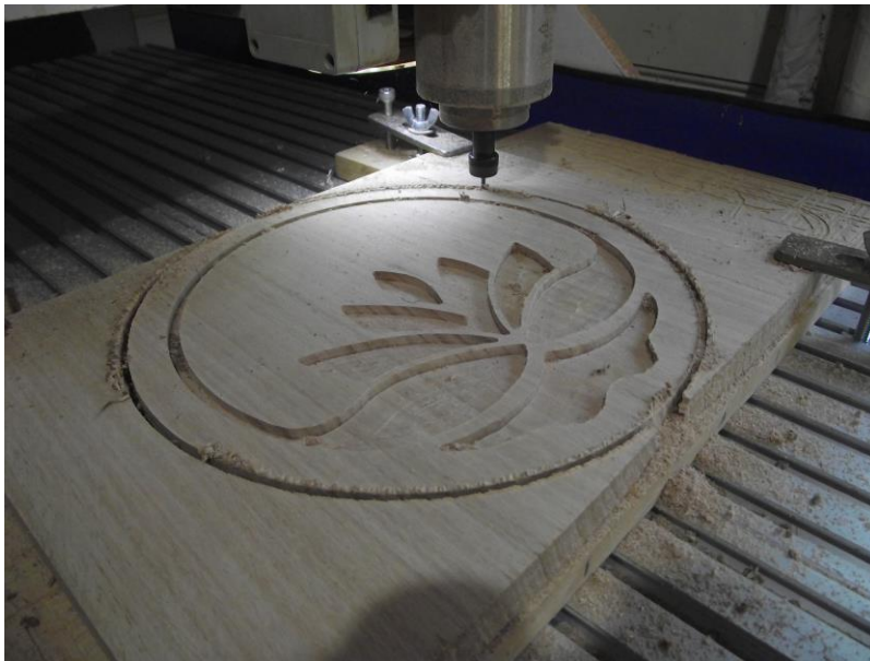
Figure 9: Machining the pockets in the substrate
