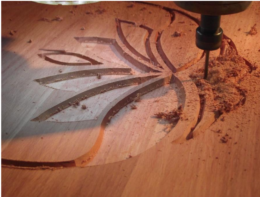
Figure 15: Clearing the substrate with the pocket MOP
