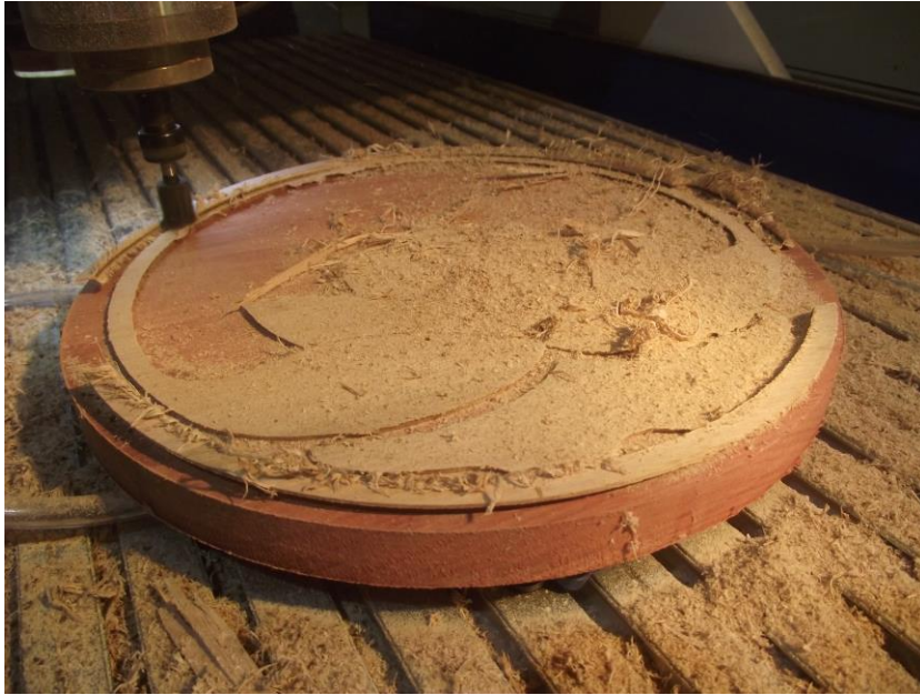
Figure 21: Clearing the top part of the inlay material.
