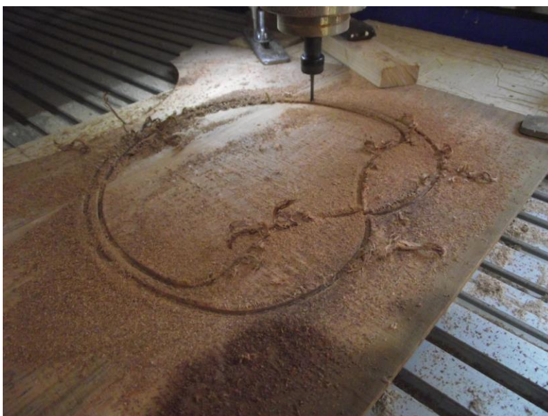
Figure 10: Machining the profiles to cut out the inlay parts
