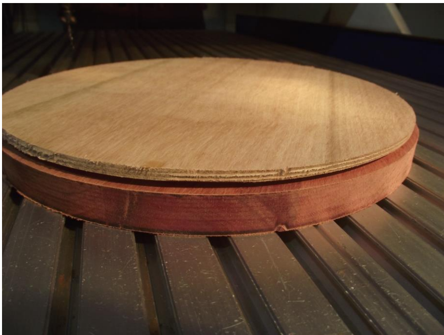
Figure 20: The Inlay glued into the substrate
