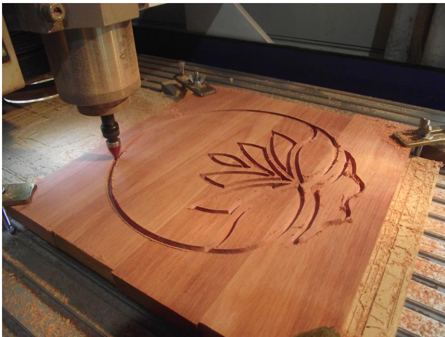
Figure 14: Cutting the V-Engrave MOP for the substrate
