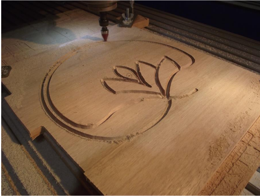
Figure 17: Cutting the V-Engrave MOP for the Inlay
